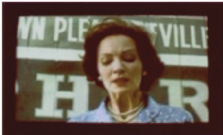
Television picture as shipped from the factory. Inaccurate color due to enhanced blue's. The reason: to emphasize "their" picture within the retail store high ambient light environment.
